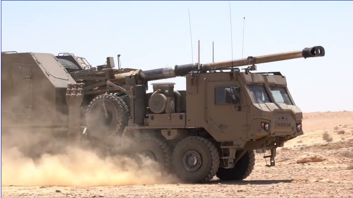
Figure 5. SIGMA 155 Roem self-propelled Howitzer used by the Israeli military whose barrel tubes are manufactured by Aubert & Duval. 52
