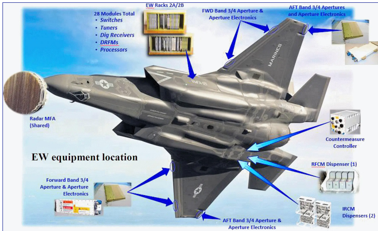
Figure 11. Location of EW equipment and EWR module. 195
